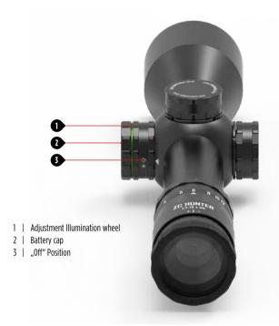
Your riflescope is featured with Automatic Illumination Management™ (AIM), which cannot be deactivated by the user. The AIM automatically deactivates the illuminated reticle if the tilt angle of the riflescope to the sides exceeds 45° and to the top or bottom exceeds 75°. The AIM also switches the illumination off automatically if it does not detect any movement for more than 2 minutes. It is automatically reactivated when movement is detected.
